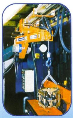
The trend towards larger centre distance and triple gob machines has meant that mould equipment has become larger and heavier.
