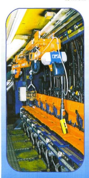
The above view is of the first installation on an 8-section 6-1/4" DG machine. The units have been readily adopted by the job change arew and the success of the installation has led to further orders by the austomer.
